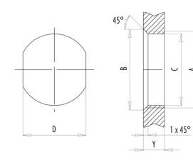
Installation direction: o-ring sits on chamfer.
